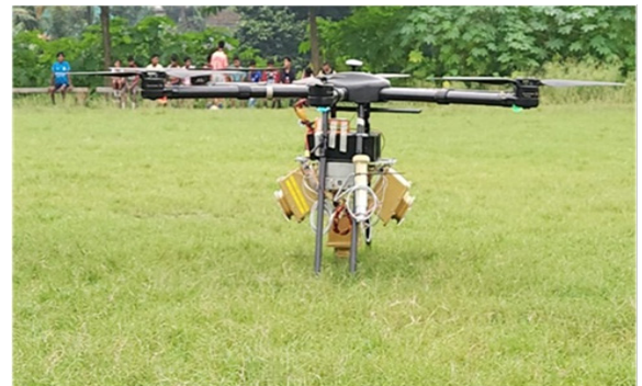
Prototype sensor payload mounted on drone platform
