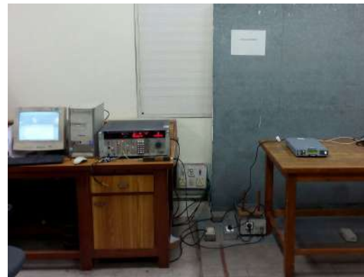
Figure 4.1: Setup for Conducted Emission Test
