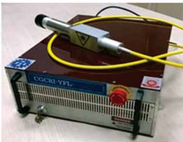
High Energy Pulsed Laser Module for Marking and engraving
