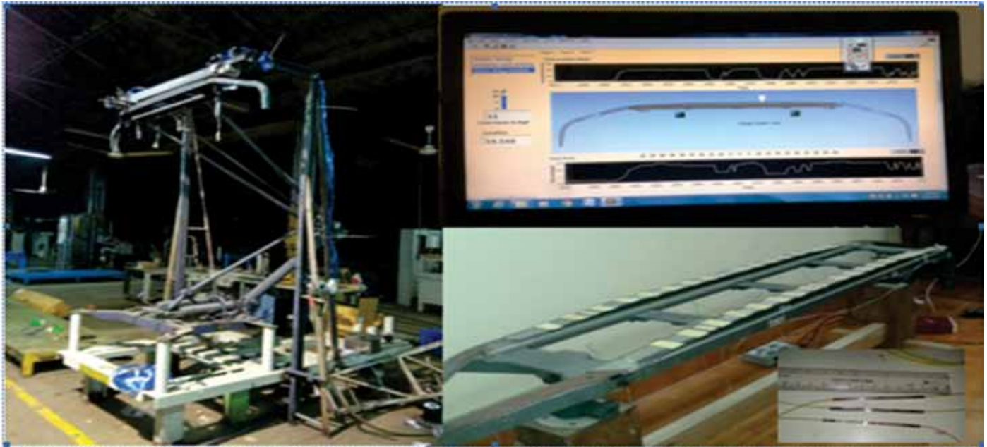
FBG sensor for condition monitoring of railway catenary-pantograph structure
