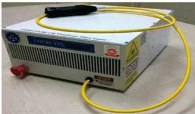
CW Laser for Stent Cutting Module
