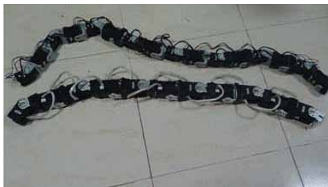
Snake Robot using Smart Actuators
