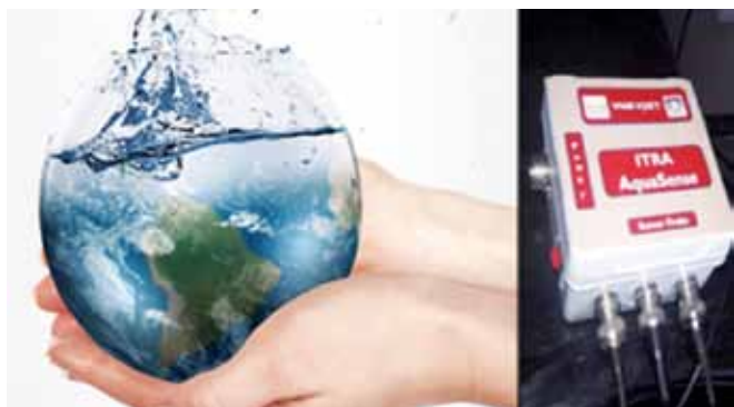
A system for sensing and wirelessly disseminating consumer water quality (contamination) and flow (leakage, the ft) information in a water distribution network
