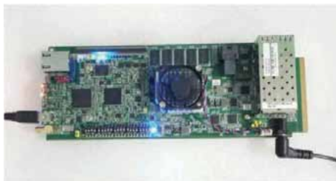
Test bed based on KeyStone C6614 Multicore SoC
