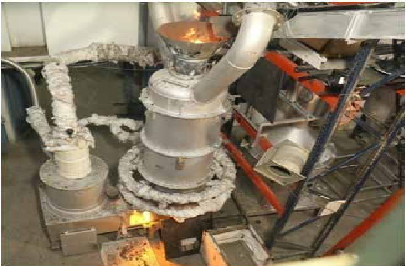
Indigenously designed and fabricated low cost furnace for smelting of PCBs.
