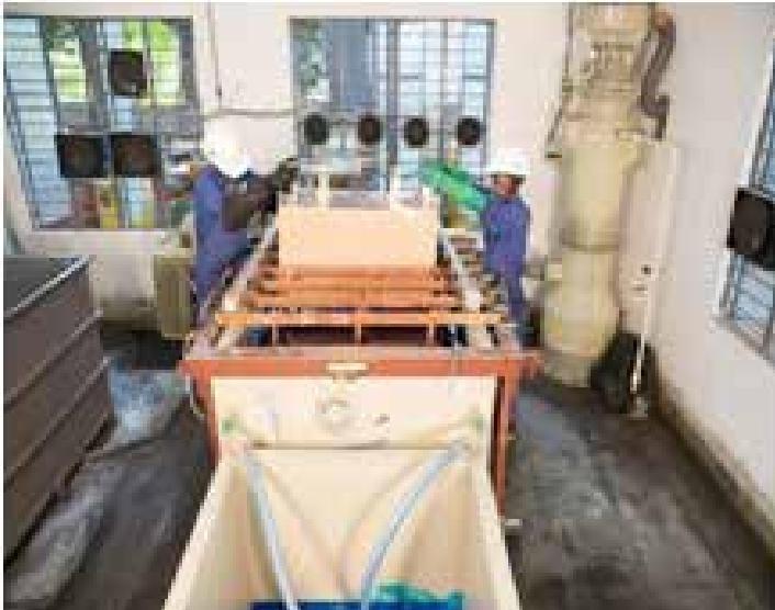
Scaled up Electrolysis of Anode Copper to 99.9% pure copper, collection of precious metals rich anode slime.
