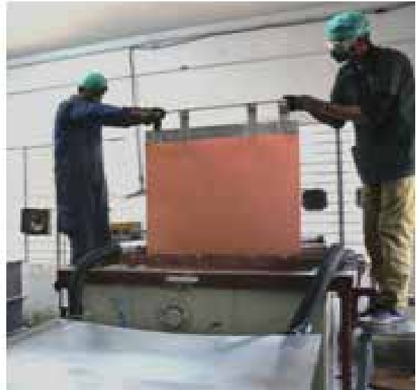
Scaled up Electrolysis of Anode Copper to 99.9% pure copper, collection of precious metals rich anode slime.
