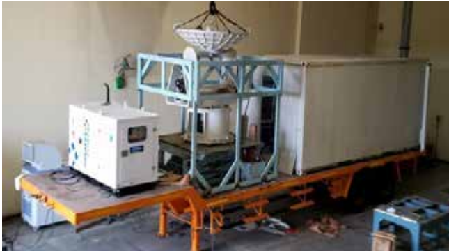
Trailer fitted with Cabin, Scissor lift with Antenna Az-El Steering pedestal and 30 kVA Diesel Generator for Ka band Cloud Radar
