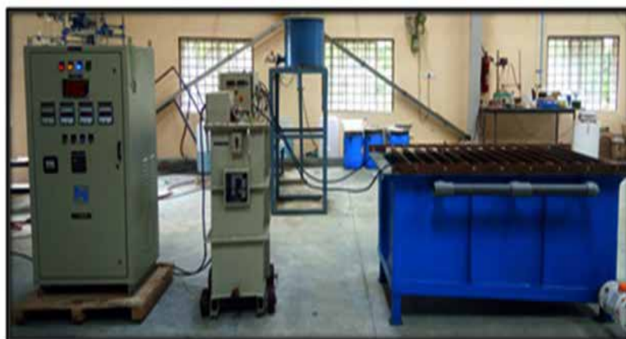
Electro-Refining unit (5kg/day Deposition rate)
