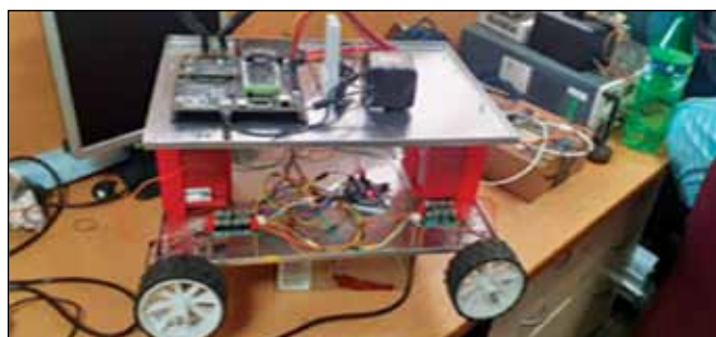
Scaled down version of the Multipurpose Agricultural Robot
