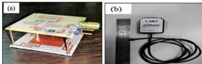
Fabricated NavIC antenna (a) coupled shorting strip (CSS) and (b) L5 ceramic antenna
