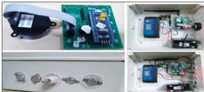
Fig. Forest Fire Wireless Sensor Node
