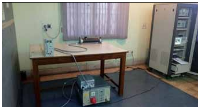
Photograph of the CE measurement set up for the DC-DC converter of M/s Urban Engineering Association.
