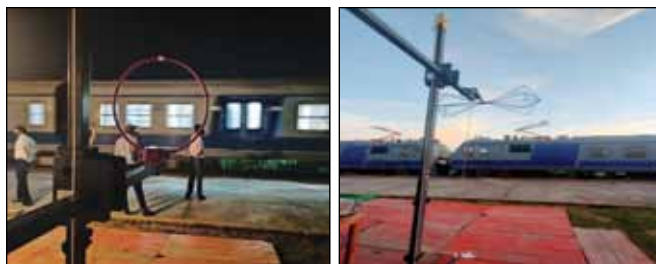
Radiated Emission measurement of MEMU train for M/s. Medha drives at Nagpur
