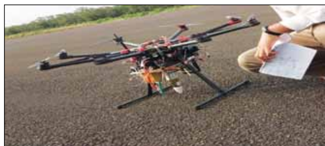
Field Testing on Octo-copter for Rocket Fuze applications
