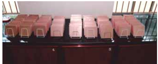
Ultra low loss MW substrates developed at C-MET through SMECH process
