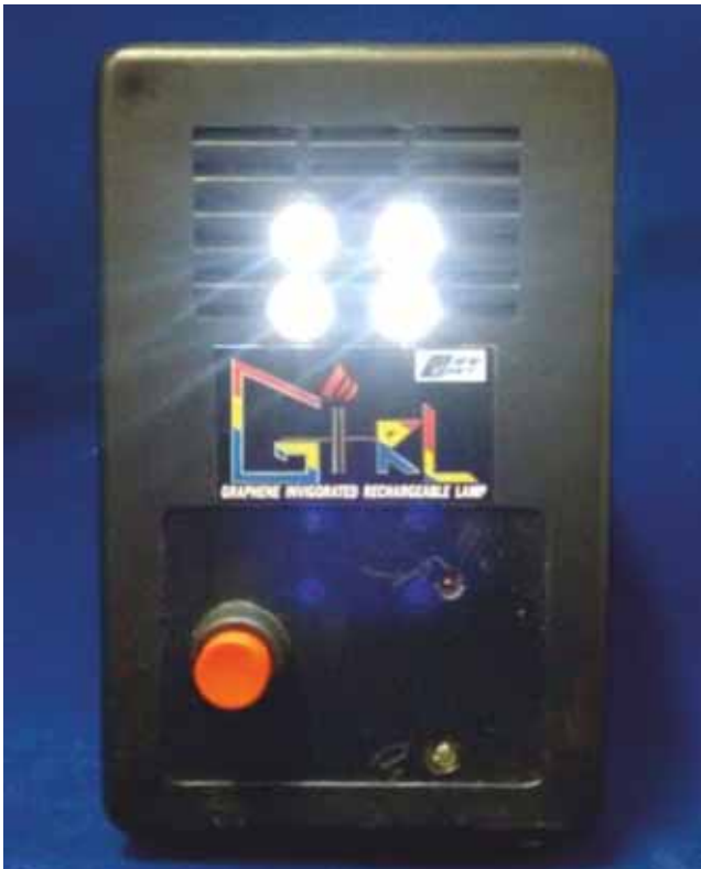
9.1 Quickly rechargeable emergency lamp
